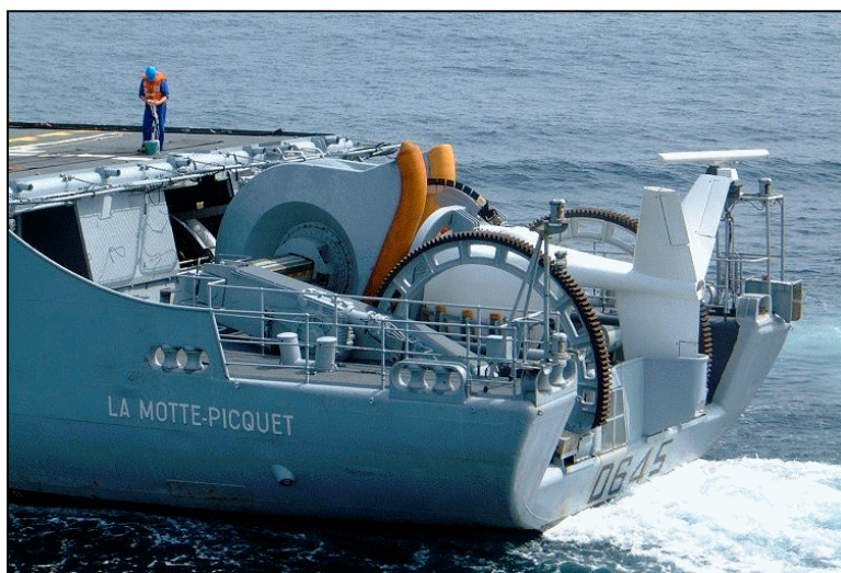
Sonar actif remorqué VDS (Variable Deep Sonar) type DUBV43C. Photo Wikipedia
